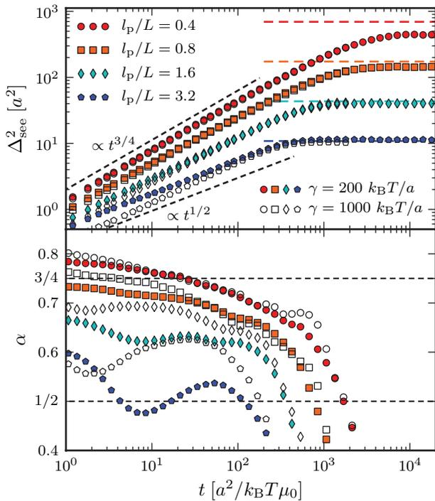
FIG. 11. Influence of stiffness  $l_p/L$  and stretching force constant  $\gamma$  on the end-to-end distance MSD [Eq. (33), upper panel] and corresponding local exponents (lower panel) in free-draining BD simulations of a polymer of length  $L = 100a$ . Results obtained with the standard stretching force constant  $\gamma = 200k_B T/a$  (filled symbols) are compared to the same observables when employing  $\gamma = 1000k_B T/a$  (open symbols).
