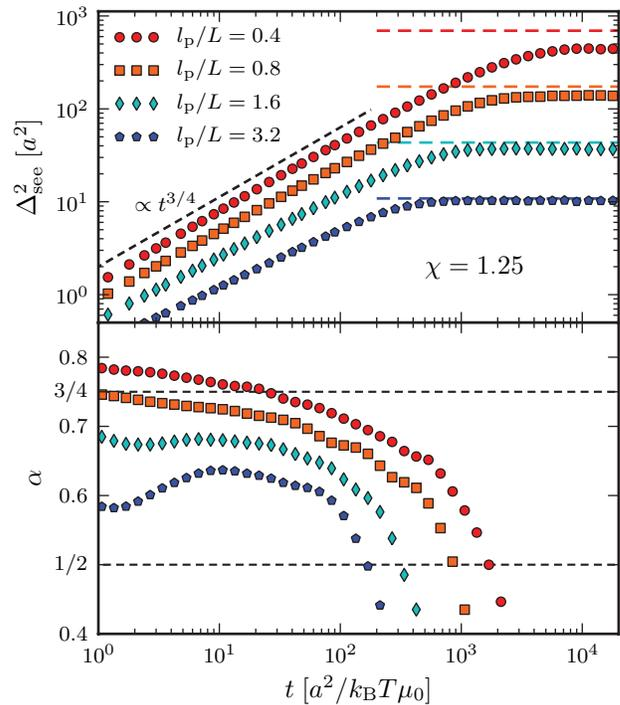
FIG. 12. (Upper panel) Influence of simultaneous variation of bending and stretching stiffness on the scalar end-to-end distance MSD [Eq. (33)] in free-draining BD simulations of a polymer of length  $L = 100a$ . Results are shown for polymers of different stiffness  $l_p/L$ , but constant  $\chi$  defined in Eq. (34), corresponding to isotropic elastic cylinders. (Lower panel) Corresponding local exponents.
