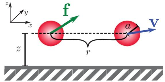
FIG. 2. Schematic illustration of the bead configuration for which the diagonal elements of the hydrodynamic interaction tensor relating the force  $\mathbf{f}$  acting on one of the beads and the velocity  $\mathbf{v}$  of the other one are plotted in Fig. 3: both spheres are located at the same height  $z$  above the no-slip wall, the vector of length  $r$  connecting the sphere centers pointing along the  $x$ -direction.
