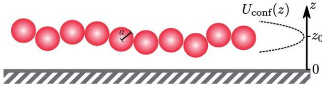
FIG. 4. Schematic illustration of the simulation setup: A polymer chain consisting of  $M$  monomers of radius  $a$  is confined by the harmonic potential  $U_{\text{conf}}$  [Eq. (17)] centered around  $z_0$  acting in the  $z$ -direction; the strength of HI varies depending on the separation  $z$  from the wall.
