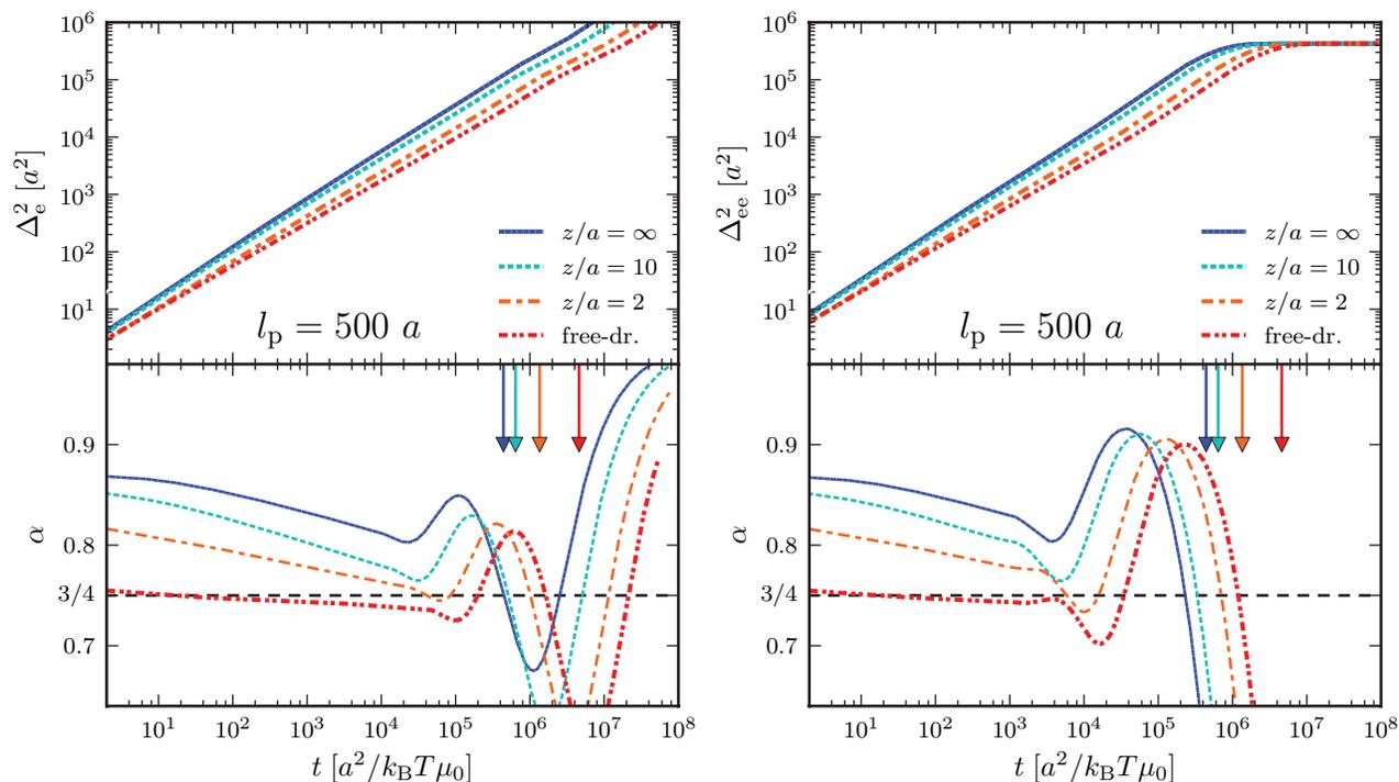
FIG. 8. MFT results for in-plane dynamics of a polymer of length  $L = 500a$  and persistence length  $l_p = 500a$ : the upper panels show the end-monomer MSD [left, Eq. (29)] and the end-to-end vector MSD [right, Eq. (30)]; the lower panels show the corresponding local exponents  $\alpha$  for various distances  $z$  from the wall as well as in the free-draining limit. Vertical arrows designate the largest MFT-relaxation times  $\Delta_1^{-1}$ .
