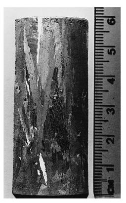
Fig. 4. A chemically etched, exterior slice of a 3 wt.% Sn-Zn ingot directionally solidified at  $1.5^{\circ}C/min$ . The dendrites that comprise the columnar crystals can be seen because of solidification shrinkage. Compare with Fig. 1.
